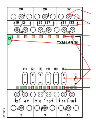
Connection terminals (No. 1 screwdriver for slotted or recessed-head \* screws) with test pickup (for 1.8...2 mm pins) and terminal number Signal designation Override status LEDs (yellow)
