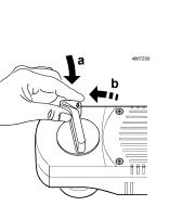
The lever is locked into position
