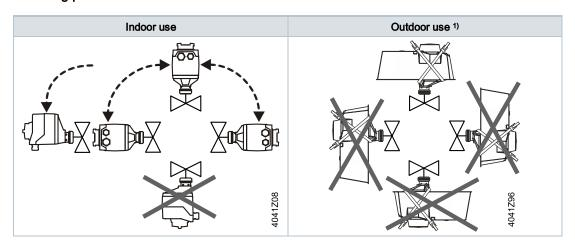
Requires the weather shield ASK39.2. Degree of protection of housing IP54 remains unchanged.
