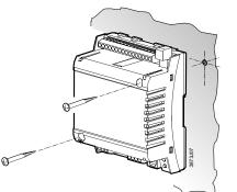
The room controllers can be mounted in any orientation, and fixed as follows:
