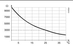
The sensor acquires the room temperature by means of its NTC resistor. The resistance value changes according to the ambient temperature. It is available for further handling by a suitable controller.
