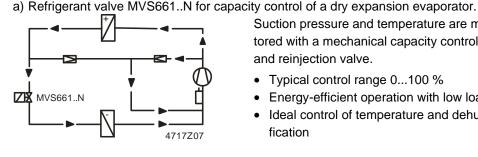
Suction pressure and temperature are monitored with a mechanical capacity controller and reinjection valve.
