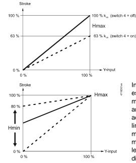
When  $k_{vs}$  reduction (DIL switch 4 in position ON) the stroke will be limited to 63 % mechanical stroke. 63 % of full stroke then corresponds to an input / output signal of 10 V. If, in addition, the stroke is limited to 80 %, for example, the minimum stroke will be
