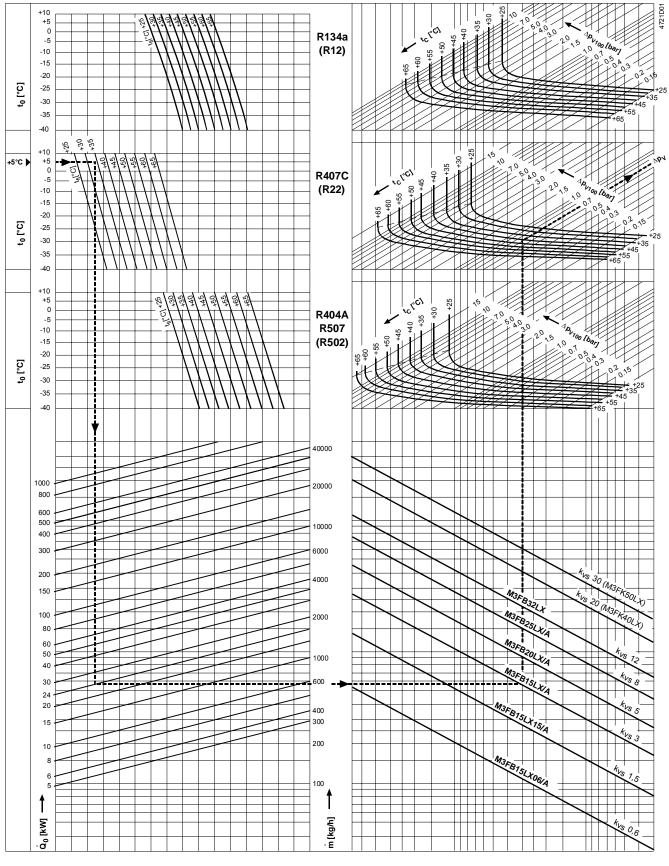
t<sub>0</sub> = Evaporation temperature [°C]
