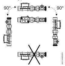
Mount the flow sensor in the return if the media temperatures exceed (>90 °C). If not possible, mount the Intelligent Valve controller remotely from the flow sensor and use the wall-mount plate EZU-WA.
