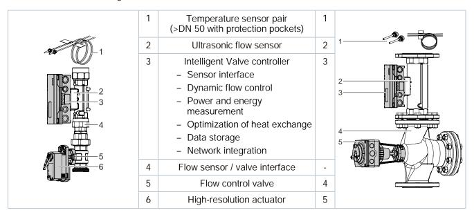
Volume flow is acquired continuously in the ultrasonic flow sensor and provided to the Intelligent Valve controller, where the controller applies it as the actual value for control or limitation by guiding the control valve position until achieving the volume flow actual value for the applicable setpoint.
