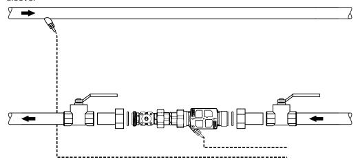
As an alternative, the sensors can be installed directly immerse in off-the-shelf ball valves with integrated measuring points (e.g. Siemens WZT-K.. / Jumo 902442/11) or t-pieces (e.g. Jumo 902442/31).
